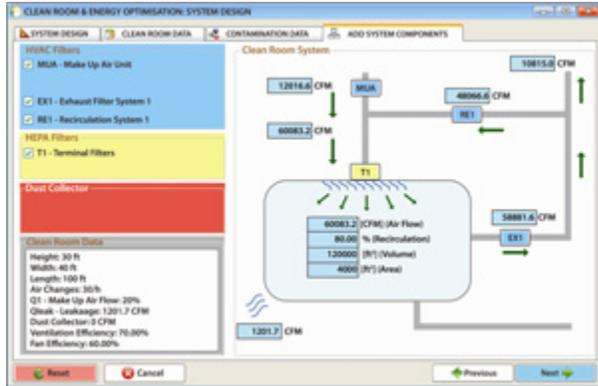
Progression screens in CREO software provide graphic representation of selections. The designer can review and make adjustments to reach the desired performance level. Image: Camfil Farr
